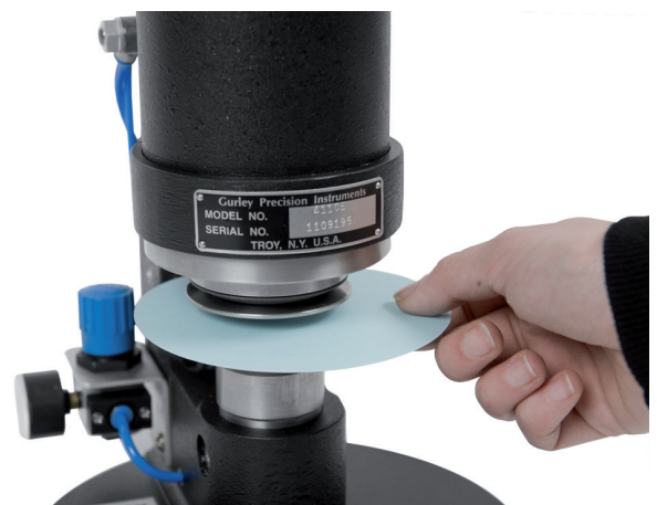
Sample is pneumatically clamped when the start button is pressed
