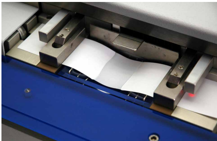
Test strip submerges in the water with pre-determined break point
