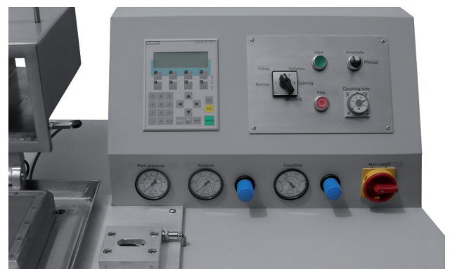
Control panel, changeable to manual control anytime
