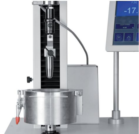
Sample support for the Ball Burst Test
