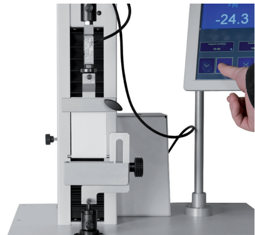
Sample support for the Wet Tensile Strength Test (Finch)
