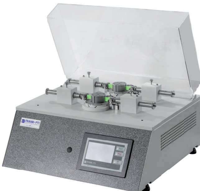
Folding unit with open security cover
