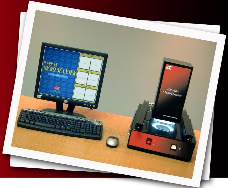
**Camera based image analyzers have superior depth of field which easily accommodate rough or poorly formed sheets.**
